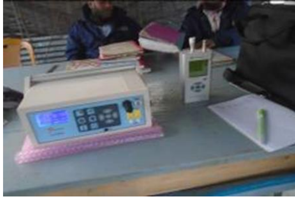
Photo 1: Respirable Dust Sampler for SPM, PM2.5, PM10 and SO2, NOx, CO measurement instruments (Combo Sampler Ecotech AAS 271Mini, India)
